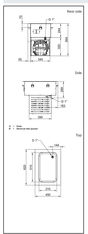
Drop-In Drop-in refrigerated well, static (1 GN container capacity)
